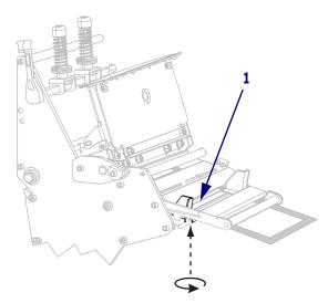
**15.** Push down the printhead assembly (1), and then rotate the printhead-open lever (2) clockwise until it locks into place.
